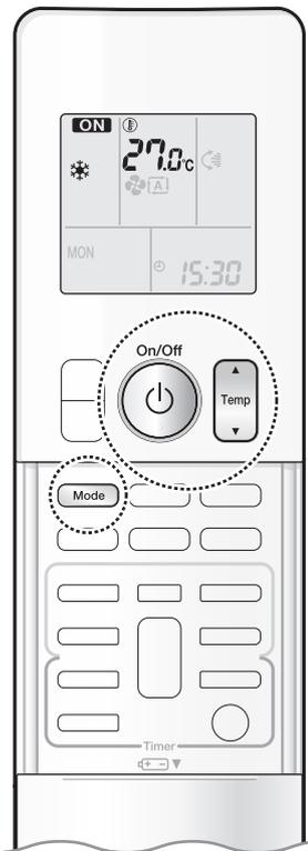
The air conditioner operates with the operation mode of your choice. From the next time on, the air conditioner will operate with the same operation mode.
