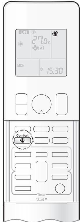
The flow of air will be in the upward direction while in COOL operation and in the downward direction while in HEAT operation, which will provide a comfortable wind that will not come in direct contact with people.
